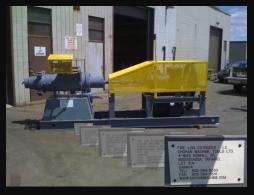
**High Speed FireLlog Extrusion Machine**
